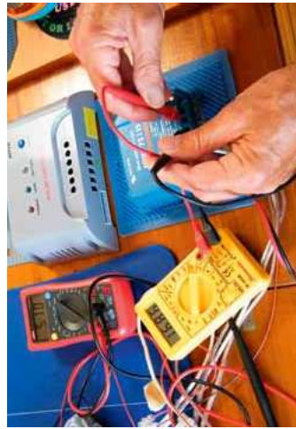
ABOVE All ready for testing. Nearest is the Sunsaver 20, then MPPT30 and Victron 75/15. The data logger recorded power on the input of the regulator. BELOW The leads from the solar panel were fed through an ammeter to the unit under test. The voltage on both input and output was taken with a digital multimeter and the output current with a second digital multimeter. Readings were taken every five minutes
