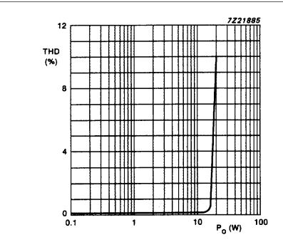
Fig.7 Total harmonic distortion (THD) as a function of output power ( $P_0$ ) for BTL application at  $R_L = 4 \Omega$ ; f = 1 kHz.
