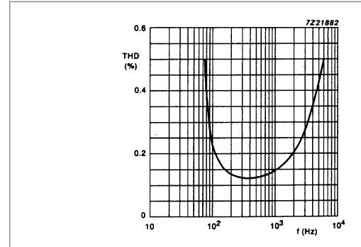
Fig.8 Total harmonic distortion (THD) as a function of operating frequency (f) for BTL application at  $R_L = 4 \Omega$ ;  $P_o = 1 \text{ W}$ .
