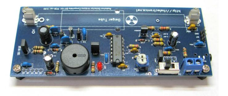
IC Socket will allow you to replace the IC easily in case you'll have any issue. Check the polarity direction of the IC. CD 4011 can be burned fast if you installed it in wrong direction.
