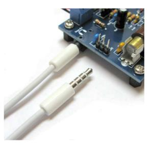
Since audio output has fixed 1ms pulse duration, we recommend to use Geiger Bot for monitoring background and testing low radiactive sources only. For high speed count please use Arduino with INT connection as described below in "Connection to MCU" section of the manual.
