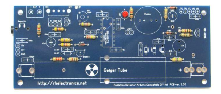
We strongly recommend you to check all resistors values with a multimeter and not rely on the color code.
