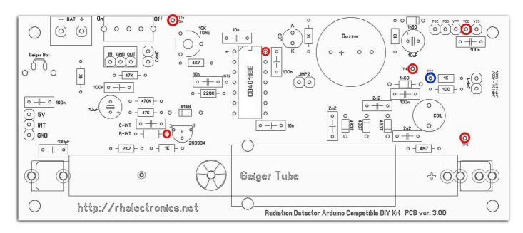
By shorting tube clips with wire you shall get one short led flash and buzzer beep. By connecting battery + to tube minus clip you shall get continuous beep.
