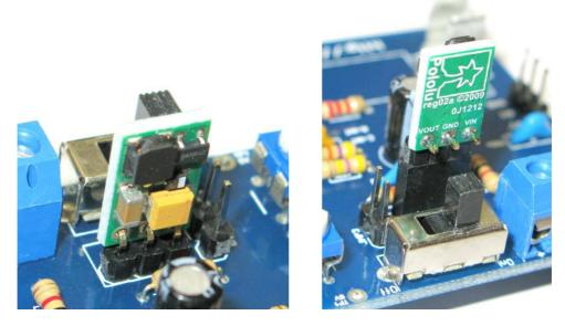
The mode can be very resonable if your enclosure is small and not allows you to use 4x1.25V Ni-MH. Different types of 5V step-up modules from Pololu, Sparkfun or eBay can be wired to the PCB. It's important to know that step up module can use the battery down to 0.8V that its not recommendable for Ni-MH discharge. That's why when using step-up its better to use alkaline batteries.
