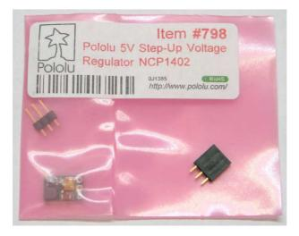
You can use 3 Pin Female Socket if you want your kit to stay configurable for different batteries, or just solder the module to the PCB directly. The board has clear marking of the module VIN, GND and VOUT direction.
