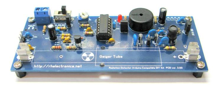
Put special attention to 1N4937 diodes, CD4011 and 2N3904 transistor polarity. We recommend you to solder 14 Pin IC Socket for the CD4011, even the photo below is missing the socket.
