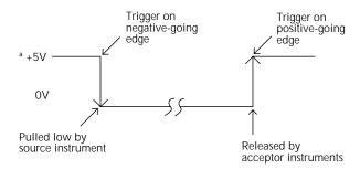
Figure 2-26 Semi-synchronous Trigger Link specifications
