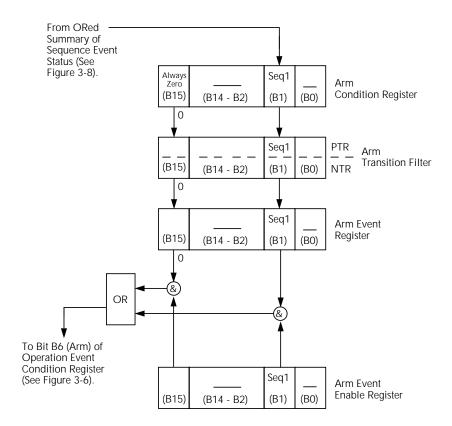
Seq 1 = Sequence 1 (Set bit indicates that the 2001 is in the arm layer of Sequence 1)
