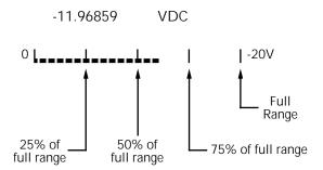
**Figure 2-1**Bar graph (zero-at-left) multiple display
