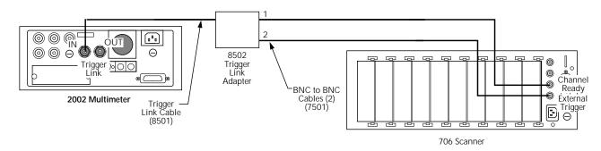
Figure 2-22 Connections using Trigger Link adapter
