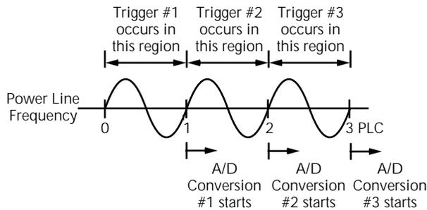
Note: A/D conversions assume an integration time of  $\leq 1$  PLC (Power Line Cycle)
