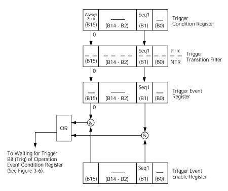
Seq 1 = Sequence 1 (Set bit indicates that the 2002 is in the trigger layer of Sequence 1)
