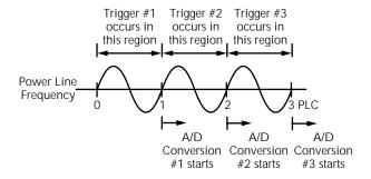
**Note:** A/D conversions assume an integration time of  $\leq$  1 PLC (Power Line Cycle)
