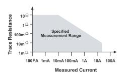
The DC in-circuit current measurement function allows a user to measure the current through a wire or a circuit board trace without breaking the circuit.
