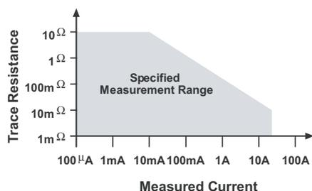
The DC in-circuit current measurement function allows a user to measure the current through a wire or a circuit board trace without breaking the circuit.
