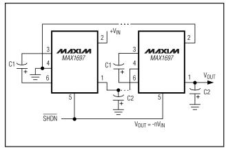
Figure 4. Cascading MAX1697s to Increase Output Voltage
