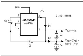
Figure 6. Combined Doubler and Inverter
