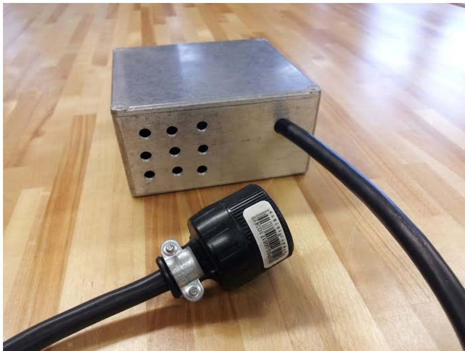
Figure 21. Convection Vents as Viewed from the Output
