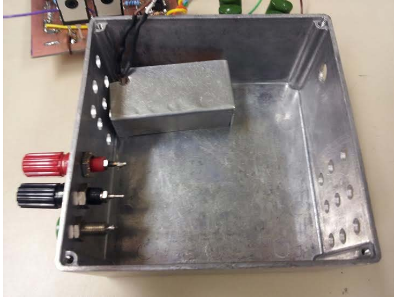
Figure 22. Inductor in Separate Aluminum Enclosure
