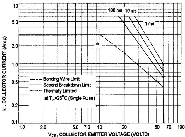
There are two limitations on the power handling ability of a transistor: average junction temperature and second breakdown. Safe operating area curves indicate  $I_C - V_{CE}$  limits of the transistor that must be observed for reliable operation, i.e., the transistor must not be subjected to greater dissipation than the curves indicate.
