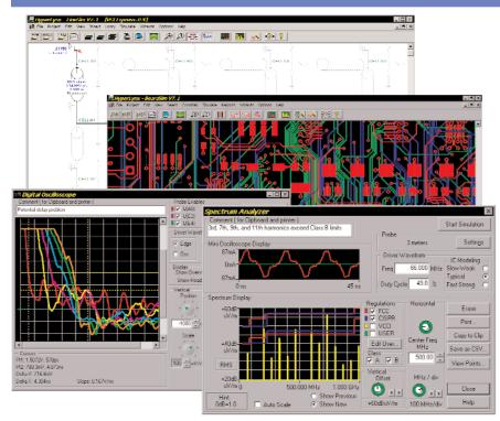
HyperLynx EXT includes a complete suite of tools for pre- and post-layout signal integrity, crosstalk and EMC analysis.
