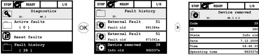
Fig. 71 Fault history menu with graphical keypad
