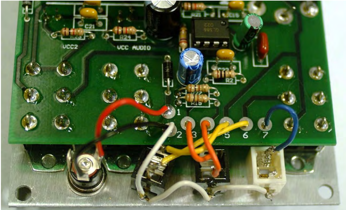
Close-up showing wires soldered to the jack tabs
