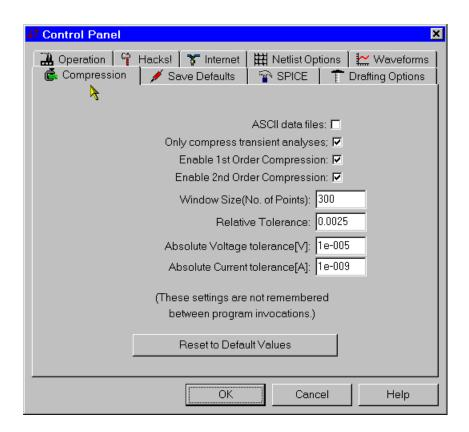
LTspice compresses the raw data files as they are generated. A compressed file can be 50 times smaller than the un-compressed one. This is a lossy compression. This
