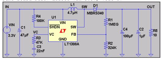
switching from 5% full load(25mA) to full load(500mA)
