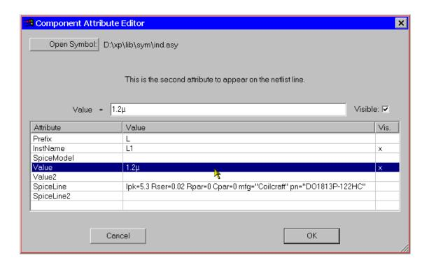
The attributes SpiceModel, Value, Value2, SpiceLine, and SpiceLine2 are all part of the overall value of the component. In terms of the way the component is netlisted for SPICE, the component will generate a line of SPICE that looks like this:
