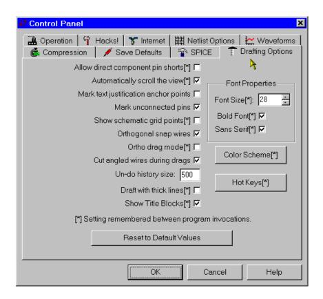
Allow direct component pin shorts: Normally you can draw a wire directly through a component and the wire segment shorting pins is deleted. If you check it, the shorting wire will not be automatically deleted.
