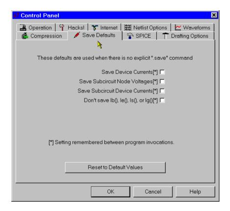
Save Device Currents: Check this so that you can plot device and terminal currents. You will also need it to be able to plot dissipation.
