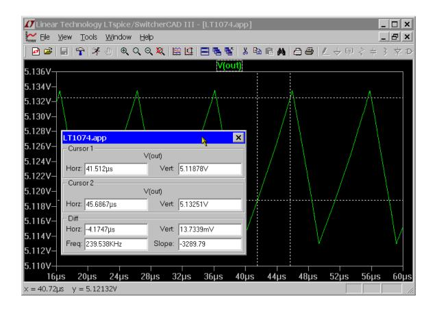
Note that there is also mouse cursor readout independent of the above attached cursor readout. As you move the mouse over the waveform window, the mouse position is readout on the status bar. If you drag the mouse as if you were going to zoom, the size of box is displayed on the status bar. This lets you quickly measure differences with the mouse cursor. If the horizontal axis is time, then this time difference is also converted to frequency.
