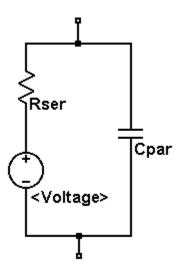
Voltage sources have historically been used as the current meters in SPICE and are used as current sensors for current-controlled elements. If Rser is specified, the voltage source can not be used as a sense element for F, H, or W elements. However, the current of any circuit element, including the voltage source, can be plotted.
