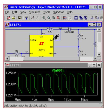
When plotting a pin current, the convention of positive current is in the direction into the pin.
