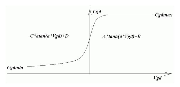
For positive Vgd, Cgd varies as the hyperbolic tangent of Vgd. For negative Vdg, Cgd varies as the arc tangent of Vgd. The model parameters a, Cgdmax, and Cgdmax parameterize the gate drain capacitance. The source-drain capacitance is supplied by the graded capacitance of a body diode connected across the source drain electrodes, outside of the source and drain resistances.
