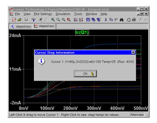
The attached cursors can also be used to readout which trace belongs to which run of a .step/.dc/.temp set of simulation runs. You can navigate the cursor from dataset to dataset with the up/down keyboard cursor keys and then right-click on the cursor to see the step information for that run.
