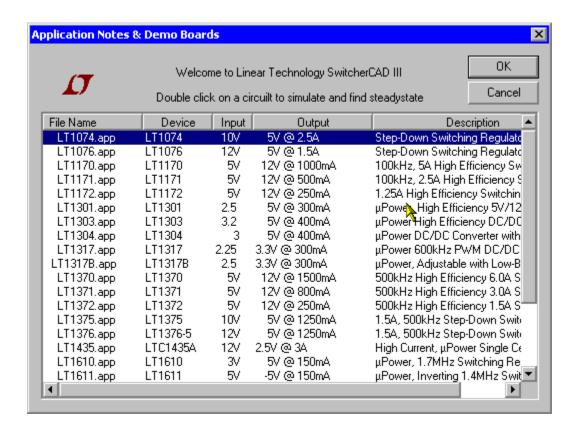
Analysis of these circuits is the same as for the synthesized circuits. This mode of operation is basically obsolete and has been replaced by the synthesized circuit mode. These circuits can be edited and modified. By default, they will be saved with a file extension of ".app" but can also be saved with a file extension of ".asc"
