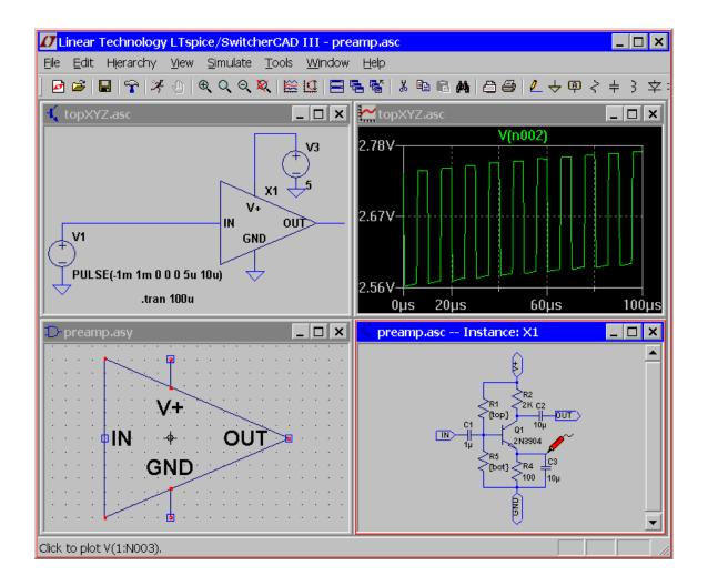
You can measure differences in this manner without performing the zoom by either pressing the Esc key or right mouse button before releasing the left mouse button.
