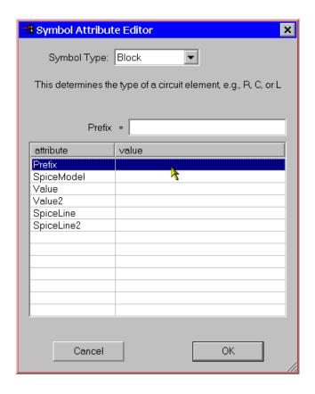
The symbol's attributes can be overridden in the instance of the symbol as a component in a schematic. For example, if you have a symbol for a MOSFET with a prefix attribute of 'M', it's possible to override the prefix to an 'X' on an instance-by-instance basis so that the transistor can be modeled as subcircuit instead.
