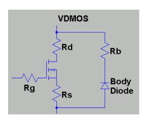
The discrete vertical double diffused MOSFET transistor(VDMOS) popularly used in board level switch mode power supplies has behavior that is qualitatively
