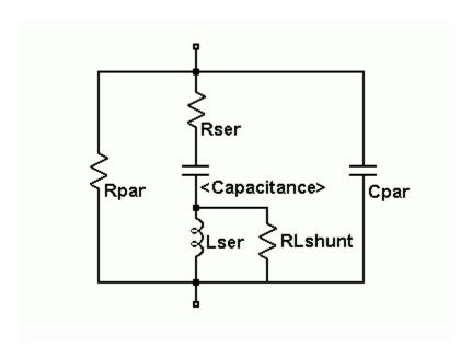
Capacitor Instance Parameters
