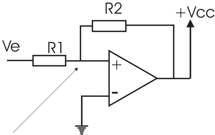
$$\frac{\frac{V_e}{R_1} + \frac{V_{CC}}{R_2}}{\frac{1}{R_1} + \frac{1}{R_2}}$$
