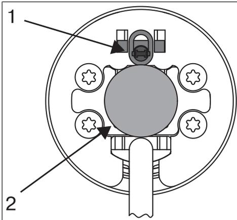
When pushed in, the mounting pin (2) locks automatically. To undo the mounting pin (2), push the tab washer (1) upwards and pull out the mounting pin (2).
