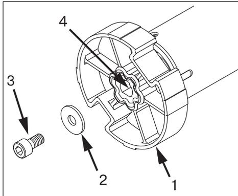
Put the drive adapter (1) onto the drive shaft of the tubular drive. For the assembly, use an M6 x 12 screw (3) with appropriate washer (2) and suitable screw retainer. Threaded hole (4)
