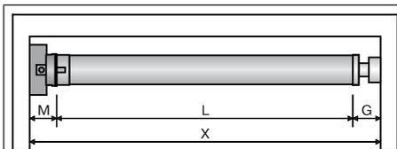
Calculate the space required at the side (M) by measuring the drive head and wall bracket. The clear dimension of the box (X) minus the space required at the side (M) and idler (G) gives the length (L) of the barrel:  $L=X-M-G$ .
