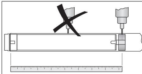
In order to secure the drive against axial displacement, we recommend screwing the drive adapter to the tube.
