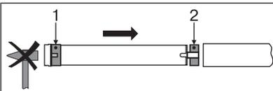
Assemble the tubular drive with the relevant thrust ring (1) and drive adapter (2). Insert the tubular drive with the pre-assembled thrust ring and drive adapter into the tube to achieve a form fit. Ensure that the thrust ring and drive adapter are secure in the tube.
