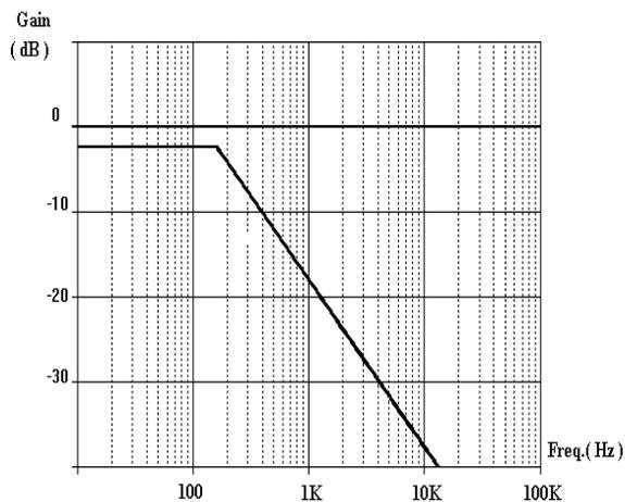
The Bode plot of the  $A_{x_{dB}}$  function shows a DC gain of -1.9dB and a pole at 163Hz.
