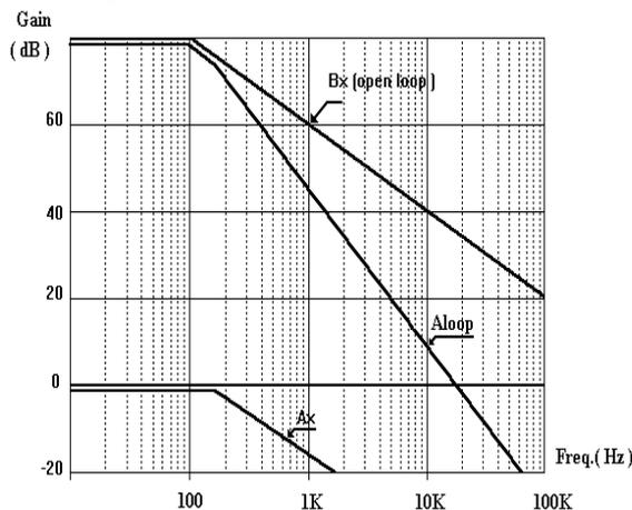
The BODE diagram shows together the error amplifier open loop transfer function, the  $A_x$  function and the resultant total  $A_{loop}$  given by the following equation :
