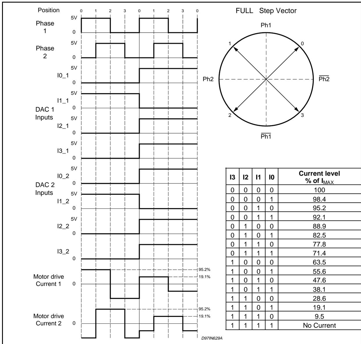
Figure 6: Half step operation mode timing diagram (Phase - DAC input and Motor Current)
