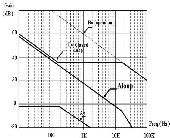
We can see that the effect of the load pole is cancelled by the zero of the Bx block ; the total Aloop cross a the 0dB axis with a slope of -20dB/decade, having in this way a stable system with an high gain at low frequency and a bandwidth of around 8KHz.
