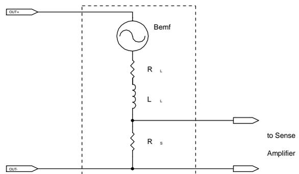
The schematic now shows the equivalent circuit of the stepper motor including a sine wave voltage generator of the Bemf. The Bemf voltage of the motor is not constant, its value changes depending on the speed of the motor.
