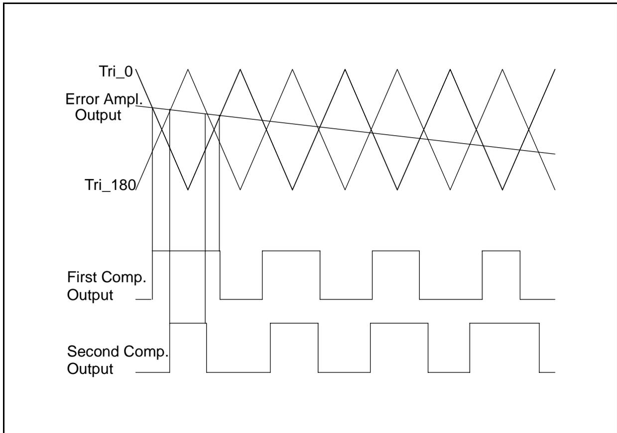
In the case of  $V_{DAC}$  equal to zero, the transconductance loop is balanced at the value of  $V_r$ , so the outputs of the two comparators are signals having the same phase and 50% of duty cycle .
