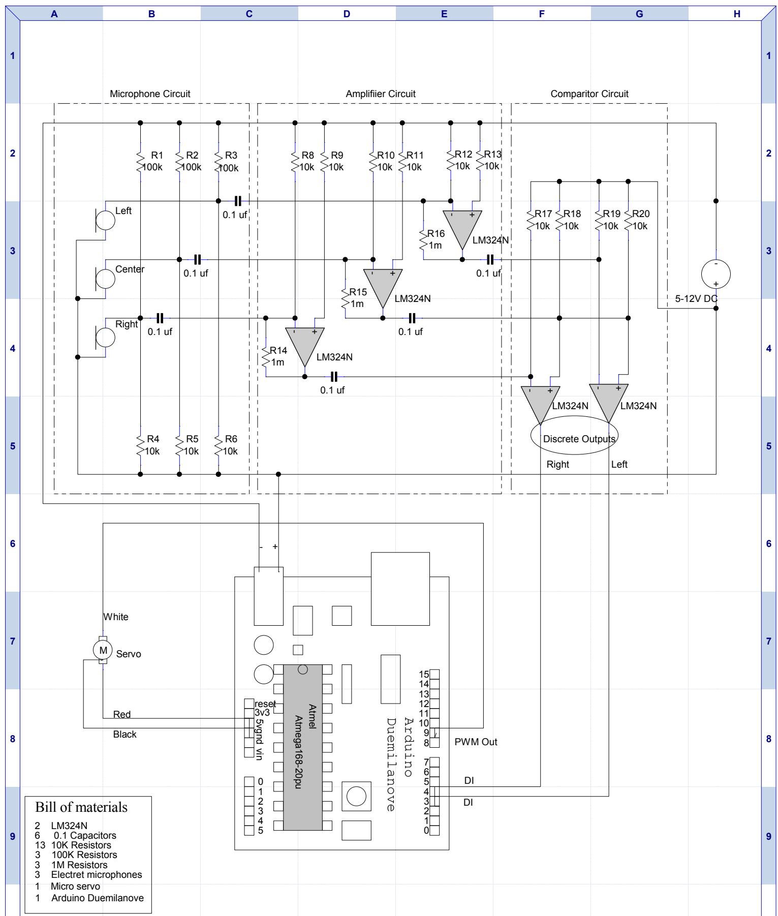
This circuit amplifies the signal from three microphones then compairs the amplitude triggering an output if the signal is louder on the left or right. These signals through the Arduino control a servo to turn a head.
