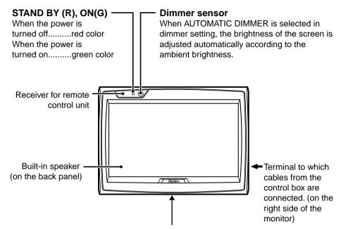
The screw hole is provided to install a TV stand at the bottom of this monitor. (1/4 inch unified screw thread, 4.5 mm of maximum length)
