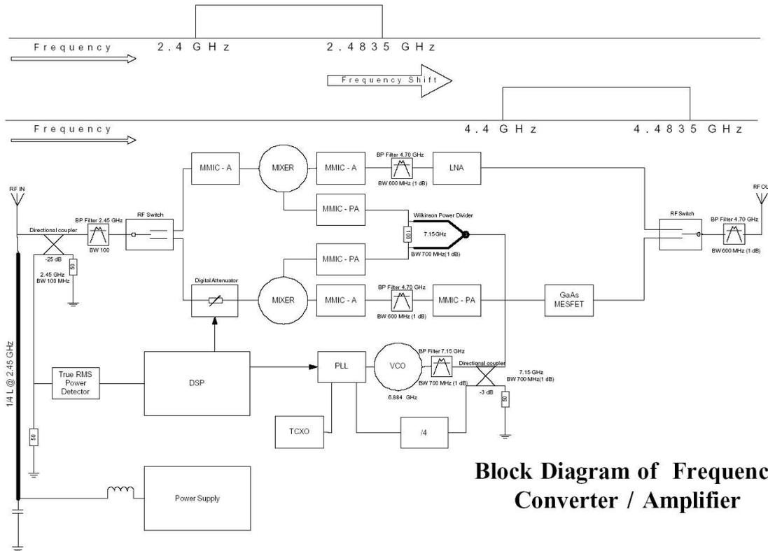
**Block Diagram of Frequency Converter / Amplifier**
