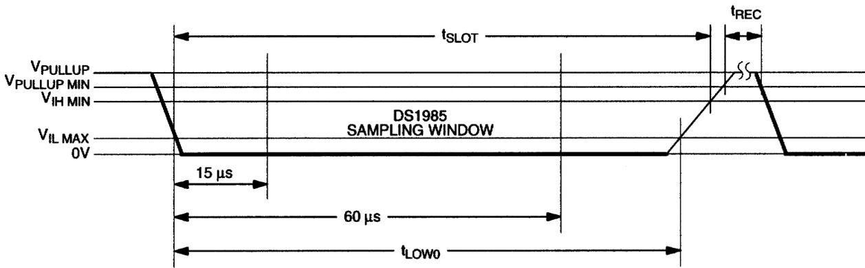
$$60 \mu s \leq t_{LOW0} < t_{SLOT} < 120 \mu s$$
