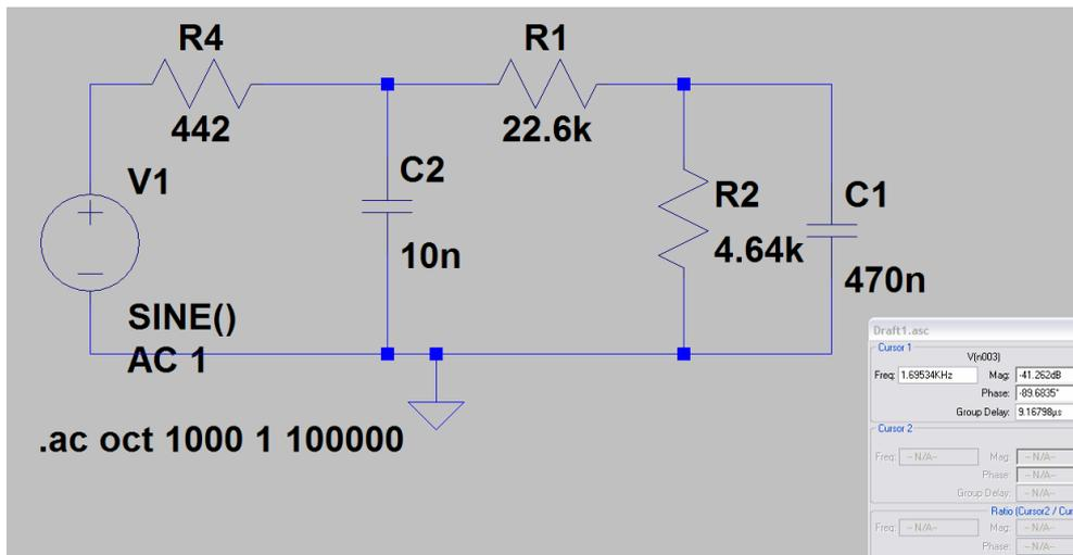
$$T = \frac{R_2}{R_1 + R_2 + R_4} \times \frac{1}{1 + p \frac{R_2}{R_1 + R_2 + R_4} \times \left( R_4 C_1 + R_1 C_1 + \frac{R_1 R_4}{R_2} C_2 \right) + \frac{R_2}{R_1 + R_2 + R_4} \times (R_1 R_4 C_1 C_2) p^2}$$
