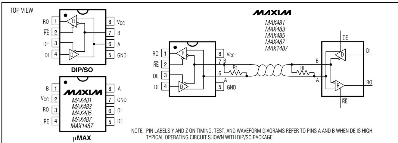
Figure 1. MAX481/MAX483/MAX485/MAX487/MAX1487 Pin Configuration and Typical Operating Circuit
