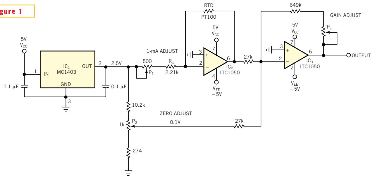
This circuit provides accurate temperature measurements using a PT100 RTD element.
