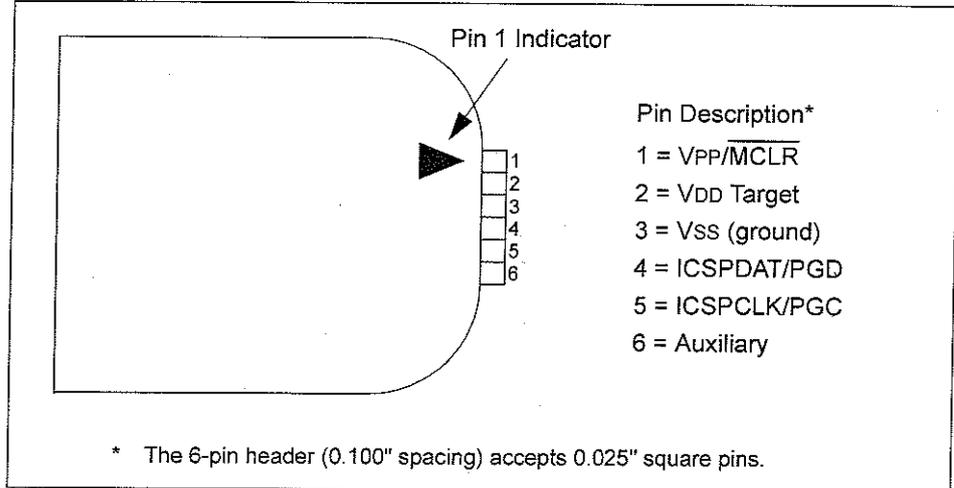
**Note:** The programming connector pin functions are different for programming Serial EEPROMS and HCS devices. See the ReadMe file ([Help>Readme](#)) included with the PICkit 2 programming software for these pinouts.
