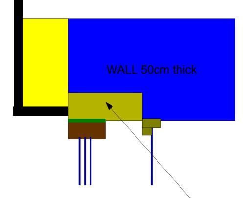
Solution #2: Rigid isolation (TMS, cellular concrete or cork panel) is Glued on the wall. Hence no thermic bridge.
