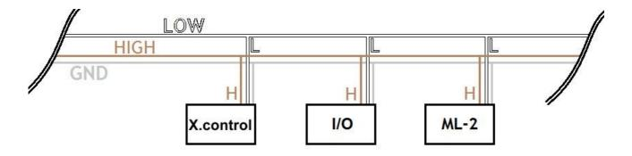
Plugging in expansion modules you need to remember to correctly set the terminator, which should be attached only at the last module throughout the system, even if the module is the only one.
