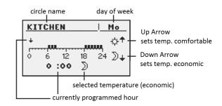
**WARNING** !!! Values of temperatures comfortable and economical are set in the "SETTINGS" menu and may be different for each of the circuits. To make the time program work, you must also enable a timed mode in the "SETTINGS" menu.
