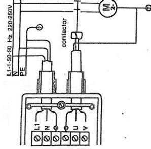
Wiring diagram for connection of single phase 220V pumps over 1.1 Kw. through remote control switch.
