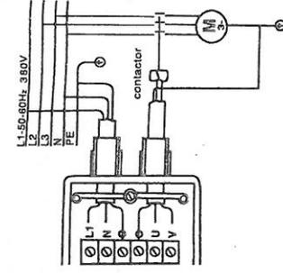
Wiring diagram for connection of three phase 380V motor pumps through remote control switch.
