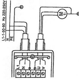
Wiring diagram for connection of single-phase 220V pumps up to 1.1 Kw.
