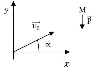
$$\text{Conditions initiales: } t=0 \quad \vec{V}_0 \left| \begin{array}{l} v_{x0} = v_0 \cos \alpha \\ v_{y0} = v_0 \sin \alpha \end{array} \right.$$
