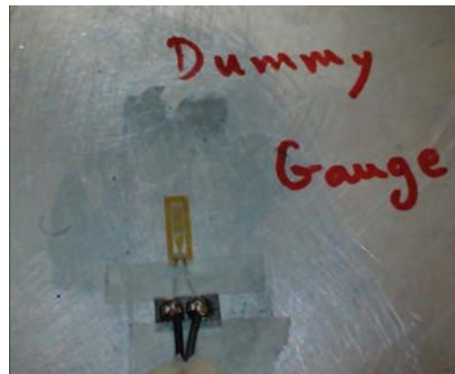
Figure 4—A dummy gauge to eliminate the thermal effect
