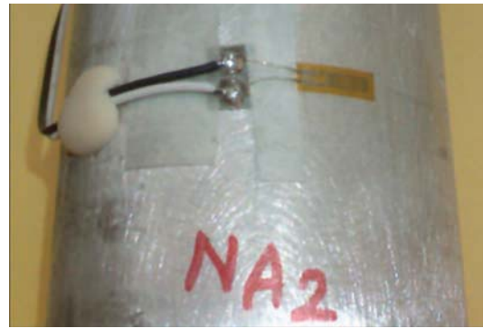
Figure 2—Electrical strain gauge on the aluminum pipe
