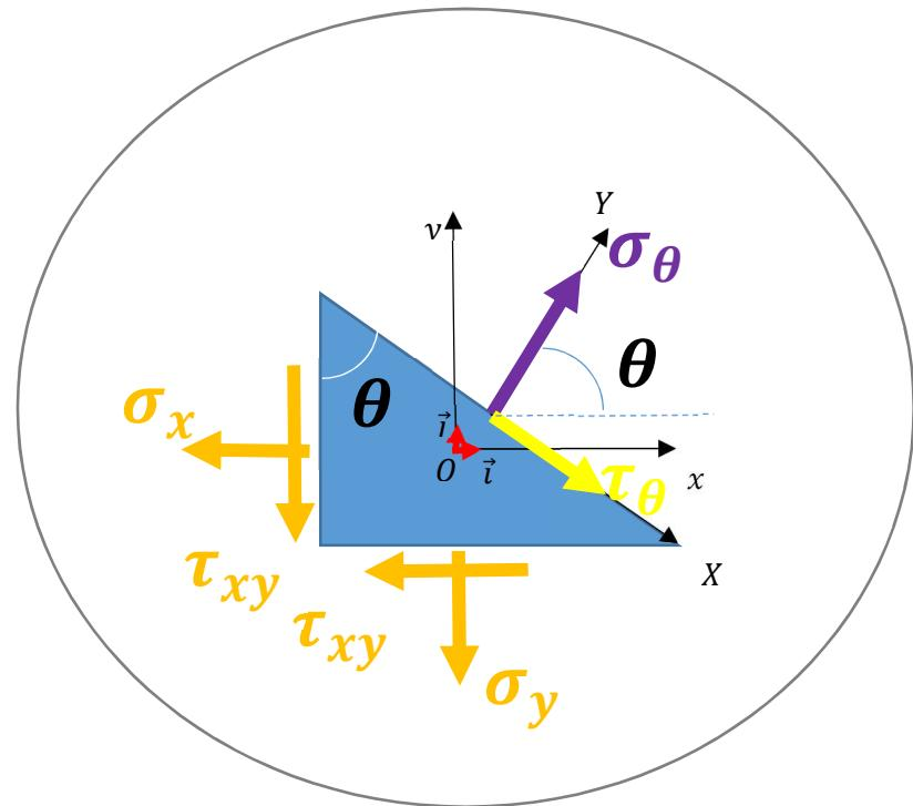
$$\tau_\theta \quad \left\{ \begin{array}{l} \sigma_\theta = \left( \frac{\sigma_x + \sigma_y}{2} \right) + \left( \frac{\sigma_x - \sigma_y}{2} \right) \cos 2\theta + \tau_{xy} \sin 2\theta \\ \tau_\theta = \left( \frac{\sigma_x - \sigma_y}{2} \right) \sin 2\theta - \tau_{xy} \cos 2\theta \end{array} \right.$$
