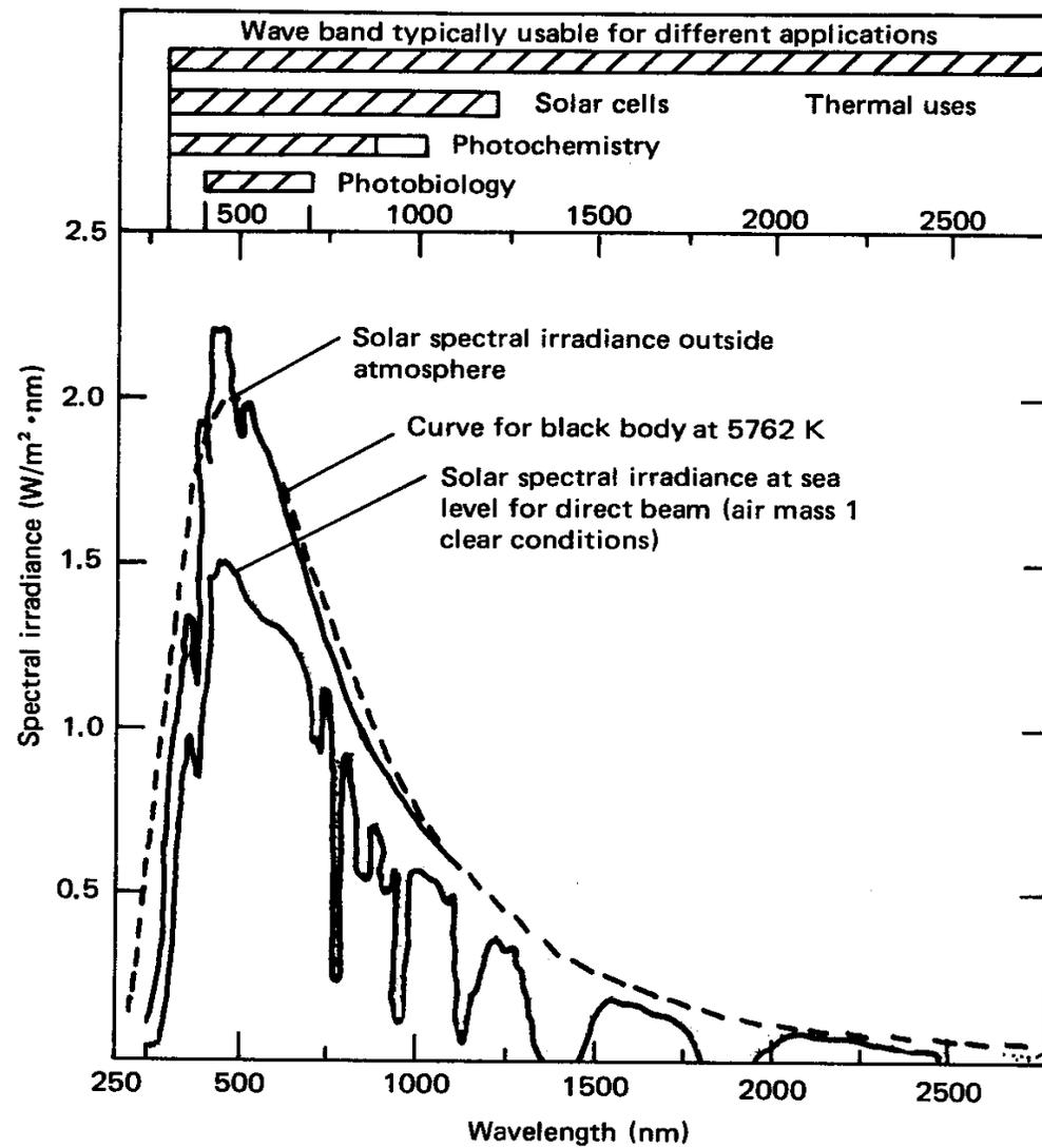
Spectral irradiance curves for direct sunlight extraterrestrially and at sea level with the sun directly overhead. Shaded areas indicate absorption due to atmospheric constituents, mainly H<sub>2</sub>O, CO<sub>2</sub>, and O<sub>3</sub>. Wavelengths potentially utilized in different solar energy applications are indicated at the top.
