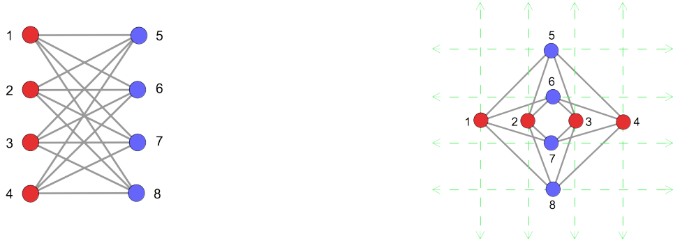
FIG. 2: The left panel illustrates the bipartate graph C_8 in column format, while the right panel illustrates the corresponding graph in cross format, often called a Chimera graph. The gray lines represent direct connections between qubits. The cross format is useful since it minimizes the number intersecting connections. The use of red and blue dots emphasize the bipartate nature of C_8 , as every red dot is connected to every blue dot, while none of the red and blue dots are connected to one another. The vertex set of C_8 is taken to be \mathcal{V}_8 = \{1, 2, \dots, 8\} and edge set is \mathcal{B}_8 = \{\{1, 5\}, \{1, 6\}, \{1, 7\}, \{1, 8\}, \{2, 5\}, \{2, 6\}, \dots, \{7, 8\}\} .
