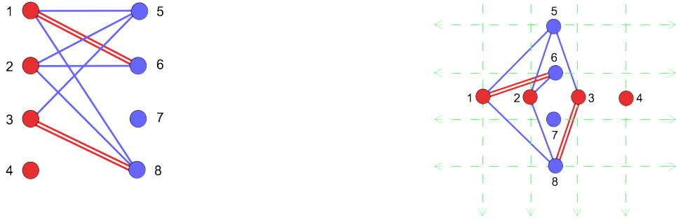
FIG. 4: The K_4 embedding onto C_8 used in our implementation of 4-bit of division on the D-Wave. The blue lines represent normal connections between qubits, while the red double-lines represent chained qubits, that is to say, qubits that are strictly correlated (and can thereby represent a single logical qubit at a higher level of abstraction). The qubits 1-6 are chained together, as are the qubits 3-8.
