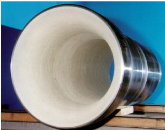
Fig. 2.18. Ceramic coating applied by a flame spray molten particle deposition method. Source: Sulzer Metco Holding A. G., Wohlen, Switzerland.
