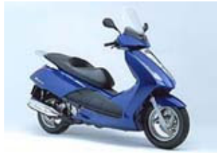
The scooter "Pantheon/Pantheon 150" (for Europe) having a water-cooled 125/150cc engine equipped with the PGM-FI
