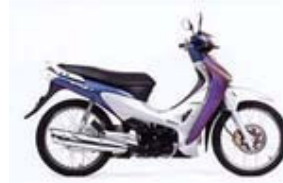
The PGM-FI (electronic fuel injection system) applied to the stylish, Super Cub type "Wave 125i" motorcycle using an air-cooled, 4-stroke, single cylinder 125cc engine (for Thailand)
